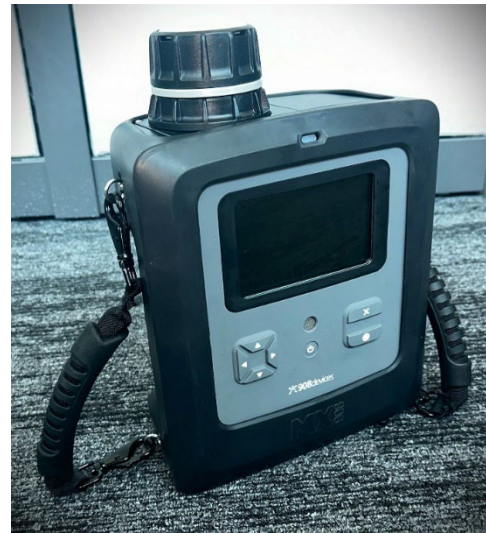
The MX908, a handheld device for real-time narcotics, explosives, and chemical detection.
