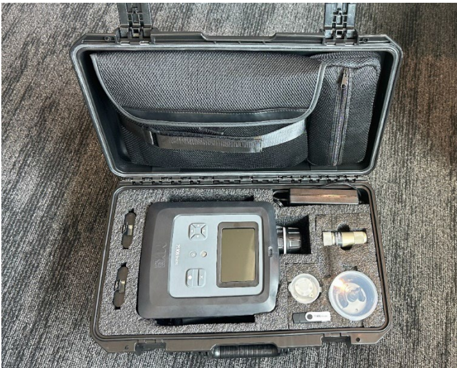
The MX908, a handheld device for real-time narcotics, explosives, and chemical detection.
